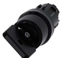
Key-operated switch O.M.R, 22 mm, round, plastic, lock number 73034, black, with 2 keys, 2 switch positions O-I, latching, actuating angle 90°, 10:30h/13:30h, key removal O+I, with laser labeling, inscription or symbol Customer-specific selection with SIRIUS ACT configurator (CIN)
