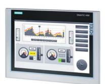
SIMATIC HMI TP1200 Comfort, Comfort Panel, touch operation, 12" widescreen TFT display, 16 million colors, PROFINET interface, MPI/PROFIBUS DP interface, 12 MB configuration memory, Windows CE 6.0, configurable from WinCC Comfort V11
