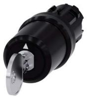
Key-operated switch BKS, 22 mm, round, plastic, lock number S1, with 2 keys, 3 switch positions I-O-II, latching, actuating angle 2x45°, 10:30h/12h/13:30h, Key removal I Z=50-unit packaging
