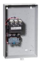
Non-reversing motor starter, Size 3, Three phase full voltage, Solid-state overload relay, OLR amp range 25-100A, 24VAC 50-60Hz coil, Non-combination type, Enclosure type 1, Indoor general purpose use, Standard width enclosure
