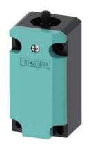
Basic switch for position switch 3SE5112 Metal enclosure 40 mm, increased corrosion protection (increased corrosion protection) according to EN 50041 Device connection 1x (M20 x 1.5) 1 NO/2 NC slow-action contacts with make-before-break without actuator head
