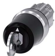
Key-operated switch IKON, 22 mm, round, metal, shiny, lock number 360012K1, with 2 keys, 3 switch positions I-O-II, latching, actuating angle  $2x45^{\circ}$ , 10:30h/12h/13:30h, Key removal I+O+II, with laser labeling, lower case
