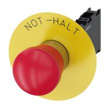
EMERGENCY STOP mushroom-type actuator, 22 mm, round, metal, shiny, red, 40 mm, positive latching, according to EN ISO 13850, pull-to-unlatch mechanism, with yellow backing plate, inscription: NOT-HALT, with holder, 1 NO+1 NC, spring-type terminal
