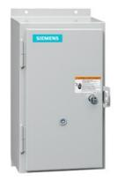
Non-reversing motor starter, Size 2 1/2, Three phase full voltage, Solid-state overload relay, OLR amp range 25-100A, 208VAC 60Hz coil, Non-combination type, Enclosure type 12, Dust/drip proof for indoors, Standard width enclosure
