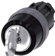
RONIS key-operated switch, 22 mm, round, plastic with metal front ring, lock number SB30, with 2 keys, 3 switch positions I>O<II, momentary contact on the left, latching on the right, actuating angle 2x45°, 10:30h/12h/13:30h, key removal O, possible special locks: SB31, 421, 455, Z=50-unit packaging
