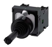
Coordinate switch, 22 mm, round, plastic, black, 2 switch positions, horizontal, momentary contact type, without mechanical interlocking in O position, with holder, 1 NO, 1 NO, screw terminal, with laser labeling, lower case
