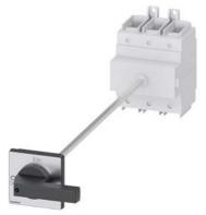
SENTRON, Switch disconnector 3FD, main switch, 3-pole, lu: 160 A, Operating power / at AC-23 A at 400 V: 75 kW, floor mounting with door coupling, knob-operated mechanism, black, 4-hole mounting of the handle
