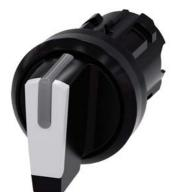
Selector switch, illuminable, 22 mm, round, plastic, white, selector switch, short, 3 switch positions I-O<II, left latching, right momentary contact type, actuating angle  $2x45^{\circ}$ , 10:30h/12h/13:30h
