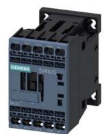
power contactor, AC-3e/AC-3, 9 A, 4 kW / 400 V, 3-pole, 220 V AC, 50 Hz / 240 V, 60 Hz, auxiliary contacts: 1 NO, spring-loaded terminal, size: S00
