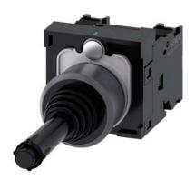
Coordinate switch, 22 mm, round, plastic with metal front ring, black, 2 switch positions, horizontal, momentary contact type, with mechanical interlocking in O position, with holder, 1 NO, 1 NO, screw terminal
