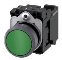
Pushbutton, 22 mm, round, plastic with metal front ring, green, pushbutton, flat, momentary contact type, with holder, 1 NO, spring-type terminal, with laser labeling, upper case and lower case, always upper case at beginning of line
