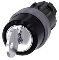
RONIS key-operated switch, 22 mm, round, plastic with metal front ring, lock number SB30, with 2 keys, 3 switch positions I>O<II, momentary contact type, actuating angle 2x45°, 10:30h/12h/13:30h, key removal O, possible special locks: SB31, 421, 455, with laser labeling, upper case and lower case, always upper case at the beginning of the word
