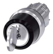
RONIS key-operated switch, 22 mm, round, metal, shiny, lock number SB30, with 2 keys, 3 switch positions >O<II, momentary contact on the left, latching on the right, actuating angle  $2x45^{\circ}$ , 10:30h/12h/13:30h, key removal O, possible special locks: SB31, 421, 455, with laser labeling, lower case
