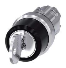
RONIS key-operated switch, 22 mm, round, metal, shiny, special lock, with 2 keys, 3 switch positions I>O<II, momentary contact on the left, latching on the right, actuating angle 2x45°, 10:30h/12h/13:30h, key removal O, possible special locks: SB31, 421, 455
