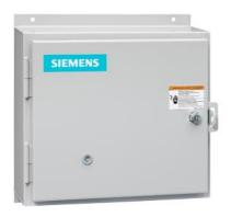
Non-reversing motor starter, Size 1, Three phase full voltage, Solid-state overload relay, OLR amp range 3-12A, Non-combination type, Enclosure type 12, Dust/drip proof for indoors, Standard width enclosure
