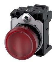
Indicator lights, 22 mm, round, plastic, red, lens, smooth, with holder, LED module, with integrated LED 230 V AC, spring-type terminal, with laser labeling, upper case and lower case, always upper case at the beginning of the word
