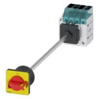
Load disconnector 3LD3, lu 25 A Main switch 3-pole + N Rated operating capacity at AC-23 A at 400V 9.0kW floor mounting Basic switch with door coupling Central hole mounting 22.5mm Toggle drive red / yellow 48x48 mm with auxiliary switch 1OE + 1S
