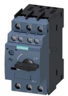
Circuit breaker size S0 for motor protection, CLASS 10 A-release 0.7...1 A N-release 13 A screw terminal Standard switching capacity with transverse auxiliary switches 1 NO+1 NC
