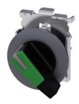
Selector switch, illuminable, 30 mm, round, Metal, matte, green, selector switch, long, front ring for flush installation, 2 switch positions O-I, latching, actuating angle 90 $^{\circ}$ , 10:30h/13:30h, Z=50-unit packaging
