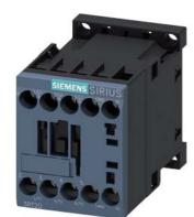
power contactor, AC-3e/AC-3, 12 A, 5.5 kW / 400 V, 3-pole, 100 V AC, 50 Hz / 100-110 V, 60 Hz, auxiliary contacts: 1 NO, screw terminal, size: S00
