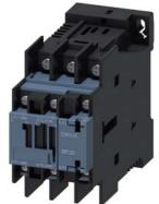
power contactor, AC-3e/AC-3, 38 A, 18.5 kW / 400 V, 3-pole, 24 V DC, auxiliary contacts: 1 NO + 1 NC, ring cable lug connection, size: S0
