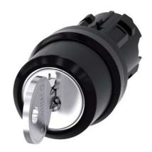
RONIS key-operated switch, 22 mm, round, plastic, lock number SB30, with 2 keys, 3 switch positions I-O-II, latching, actuating angle 2x45°, 10:30h/12h/13:30h, key removal O, possible special locks: SB31, 421, 455, with laser labeling, upper case and lower case, always upper case at beginning of line
