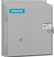
Reversing motor starter, Size 1, Three phase full voltage, Solid-state overload relay, OLR amp range 0.25-1A, Non-combination type, Enclosure type 4X fiberglass, Water/dust tight noncorrosive, Standard width enclosure
