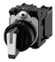
Selector switch, illuminable, 22 mm, round, plastic, white, selector switch, short, 3 switch positions I-O-II, latching, 10:30h/12h/13:30h, with holder, 1 NO, 1 NO, screw terminal
