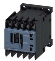
power contactor, AC-3e/AC-3, 12 A, 5.5 kW / 400 V, 3-pole, 24 V DC, 0.7-1.25\* Us, with integrated varistor, auxiliary contacts: 1 NC, ring cable lug connection, size: S00
