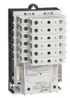
Electrically held lighting contactor, (convertible to mech. held), Amp rating 30A (tungsten 20A), 6 N.C. / 3 N.O. poles, 277V 60Hz / 240V 50Hz coil, Noncombination type, Enclosure NEMA type (open), No enclosure
