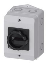
SENTRON, Switch disconnector 3LD, main switch, 3-pole, lu: 32 A, Operating power / at AC-23 A at 400 V: 11.5 kW, molded-plastic encapsulation for inch cable gland, 1 NC, 1 NO, rotary operating mechanism, black
