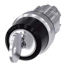
RONIS key-operated switch, 22 mm, round, metal, shiny, Lock No. 421, with 2 keys, 3 switch positions I-O-II, latching, actuating angle 2x45°, 10:30h/12h/13:30h, Key removal I+O+II, with laser labeling, inscription or symbol Customer-specific selection with SIRIUS ACT configurator (CIN)
