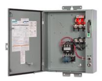
Pump control panel, Size 2, Three phase full voltage, Solid-state overload relay, OLR amp range 13-52A, 220-240/440-480VAC 60Hz coil, Standard type contactor, 100A fusible disconnect, 100A/600V fuse clip, HOA Sel Sw. <(>&<)> Start P.B., Enclosure NEMA type 3/3R, Weather proof outdoor use
