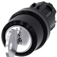
RONIS key-operated switch, 22 mm, round, plastic, lock number SB30, with 2 keys, 3 switch positions I-O-II, latching, actuating angle 2x45°, 10:30h/12h/13:30h, Key removal I+II, possible special locks: SB31, 421, 455, with laser labeling, upper case
