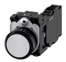
Pushbutton, 22 mm, round, plastic, gray, pushbutton, flat, momentary contact type, with holder 1 NO+1 NC, screw terminal, with laser labeling, upper case and lower case, always upper case at beginning of line
