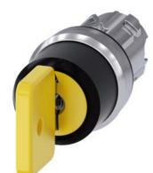
Key-operated switch O.M.R, 22 mm, round, metal, shiny, lock number 73033, yellow, with 2 keys, 3 switch positions I>O<II, momentary contact on the left, latching on the right, actuating angle 2x45°, 10:30h/12h/13:30h, Key removal II, with laser labeling, upper case
