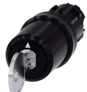
key-operated switch Siemens, 22 mm, round, plastic, lock number SSG10, with 2 keys, 3 switch positions I>O<II, momentary contact on the left, latching on the right, actuating angle 2x45°, 10:30h/12h/13:30h, key removal O, with laser labeling, lower case
