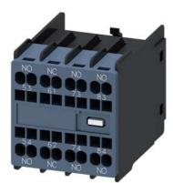
auxiliary switch, on the front, 3 NO + 1 NC, 53/54, 61/62, 73/74, 83/84, current path: 1 NO, 1 NC, 1 NO, 1 NO, spring-loaded terminal, physically coded, only with contactor relays 3RH2140 and 3RH2440 combinable (according to EN 50011)
