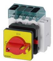
Load disconnector 3LD3, lu 63 A Main switch 3-pole + N Rated operating capacity at AC-23 A at 400V 22.0 kW Front plate mounting Basic switch with Central hole mounting 22.5mm Toggle drive red / yellow 48x48 mm with auxiliary switch 10E + 1S
