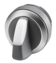
Selector switch for extension units, 22mm, round, plastic, latching, with integrated white LED (illuminable), 3 switch positions 1-0-2, 2 NO contacts. (incl. PCB, contact module)
