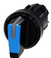
Selector switch, illuminable, 22 mm, round, plastic, blue, selector switch, short, 3 switch positions I>O<II, momentary contact on the left, latching on the right, actuating angle  $2x45^{\circ}$ , 10:30h/12h/13:30h
