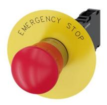
EMERGENCY STOP mushroom pushbutton, 22 mm, round, metal, shiny, red, 40 mm, positive latching, acc. to EN ISO 13850, rotate-to-unlatch, with yellow backing plate, inscription: EMERGENCY STOP, with holder, 1 NO+1 NC, screw terminal
