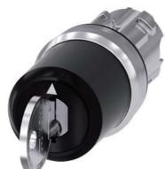
Key-operated switch IKON, 22 mm, round, metal, shiny, lock number 360012K1, with 2 keys, 3 switch positions I-O-II, latching, actuating angle 2x45°, 10:30h/12h/13:30h, Key removal I+O+II, Z=50-unit packaging
