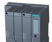
SCALANCE XF204 managed two BusAdapters BA 2xRJ45 HA IEC 62443-4-2 certified; IE switch, 4 x 10/100 Mbps, 2 x BusAdapter interface, error signaling contact, set pushbutton, redundant 24 V DC power supply, PROFINET device, extended temperature range -40 °C...+70 °C, conformal coating, with electronic manual on DVD, C-PLUG optional, delivery with BusAdapter. preassembled 6DL1193-6AR00-0AA0
