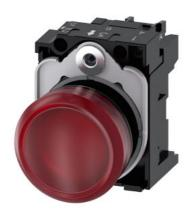
Indicator light, 22 mm, round, plastic, red, lens, smooth, with holder, LED module, with integrated LED 24 V AC/DC, screw terminal, with laser labeling, upper case and lower case, always upper case at beginning of line
