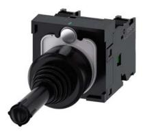
Coordinate switch, 22 mm, round, plastic, black, 2 switch positions, vertical, momentary contact type, without mechanical interlocking in O position, with holder, 1 NO, 1 NO, screw terminal, with laser labeling, upper case and lower case, always upper case at beginning of line
