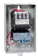
Non-reversing motor starter, Size 00, Three phase full voltage, Solid-state overload relay, OLR amp range 0.75-3.4A, 208VAC 60Hz coil, Non-combination type, Enclosure type 1, Indoor general purpose use, Standard width enclosure
