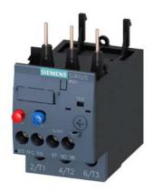
Overload relay 17...22 A Thermal For motor protection Size S0, Class 10 Contactor mounting Main circuit: Screw Auxiliary circuit: Screw Manual-Automatic-Reset
