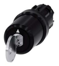
key-operated switch Siemens, 22 mm, round, plastic, lock number SSG10, with 2 keys, 3 switch positions I>O<II, momentary contact on the left, latching on the right, actuating angle 2x45°, 10:30h/12h/13:30h, key removal O Z=50-unit packaging
