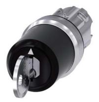
Key-operated switch IKON, 22 mm, round, metal, shiny, lock number 360012K1, with 2 keys, 3 switch positions I-O-II, latching, actuating angle 2x45°, 10:30h/12h/13:30h, Key removal I+O+II
